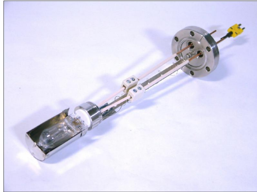
1Kw I.R. heater with K thermocouple and inconel screen
